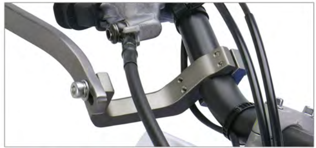
Removed sharp edge to reduce cable damage.
