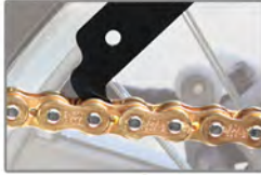
A. Lightly attach Chain Checker on the chain roller.
