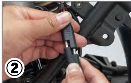
Connect the battery charging connector and the terminal unit connector.
