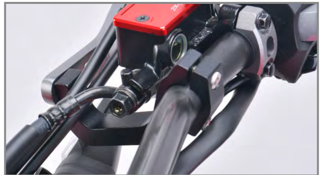
Special U-clamp that greatly avoids interference between the master cylinder and wiring.
