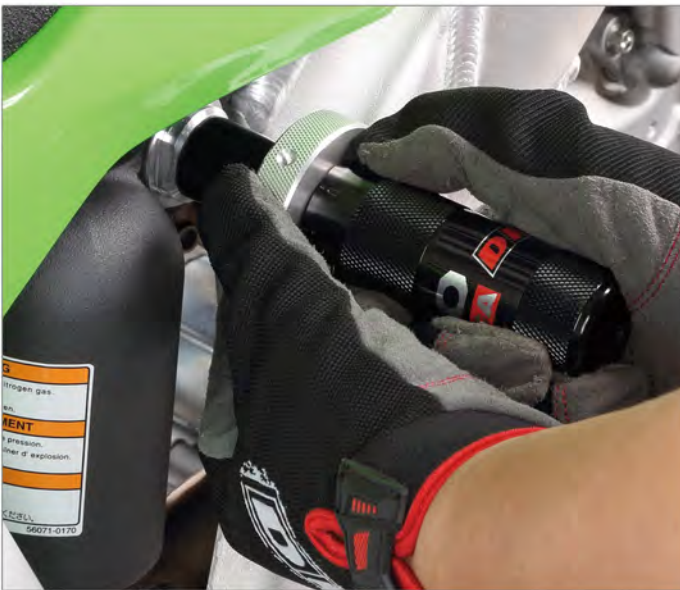
Spacer: A spacer is included. The KYB / SHOWA fork (φ59.2 mm) fork can be clamped when the spacer is installed, and the WP (clamp diameter φ60 mm) fork can be clamped when the spacer is removed.
