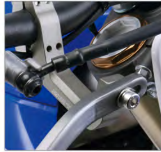
Removed sharp edge to reduce cable damage.
