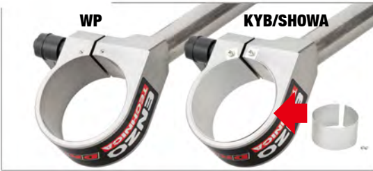
Spacer: A spacer is included. The KYB / SHOWA fork (φ59.2 mm) fork can be clamped when the spacer is installed, and the WP (clamp diameter φ60 mm) fork can be clamped when the spacer is removed.
